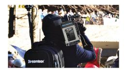
The Streambox Avenir Mini 2 is a new and improved HD/SD mobile broadcasting and streaming video encoder with integrated modems, which bond multiple IP networks at once including: 3G/4G, Wi-Fi, SNG, BGAN, Internet and Ethernet.
