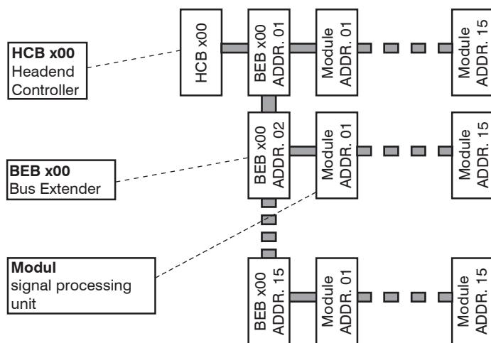
The number of the possible module connections (00 ... 15) to a BEB x00 depends on the total power consumption of this line.
