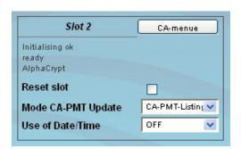
Individual CA modules must be initialized before setting the CA services. For this purpose the box "Reset slot" is clicked. The mode of the CA-PMT update will be adjusted on the next line. You can select between CA and CA-PMT PMT-list entry, where the latter is not supported by all CAM's.
