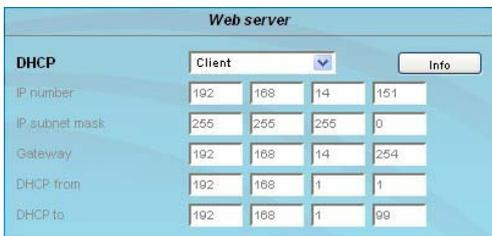
If the device is set to "DHCP-Client", it automatically obtains an IP address from the DHCP server on the network. The manual network settings are grayed out and are therefore disabled.
