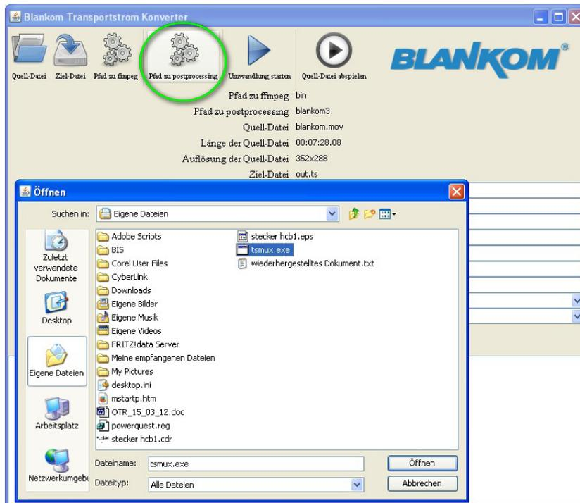
After the successful completion of the installation of the playback tool, you can select video converter already in a file. In the following, a video file is selected and clicked "Quell-Datei abspielen". This will open the video player and returns the selected file.
