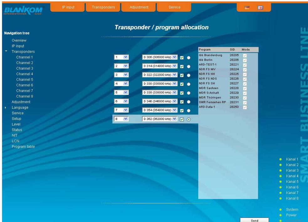
To make changes, first the desired channel is to be selected. This is done either by clicking the appropriate selector outside right next to the output channel in the middle of the channel list or by clicking on "Channel" in the navigation tree on the left side, which is listed as a submenu of the menu "Transponders".
