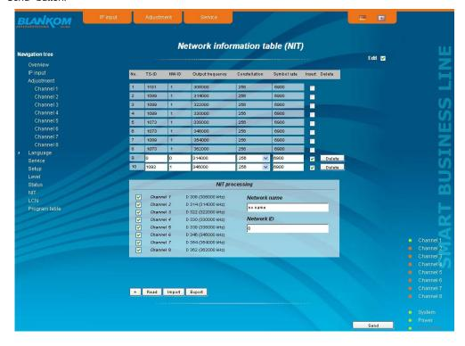
For changes of the NIT is to be noted that these changes must be made in the NIT of each module. It is therefore recommended to prefer the automatic NIT processing of the manual NIT processing.
