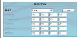
If the module is set to "DHCP-Client", it automatically obtains an IP address from the DHCP server on the network. The manual network settings are grayed out and are therefore disabled.
