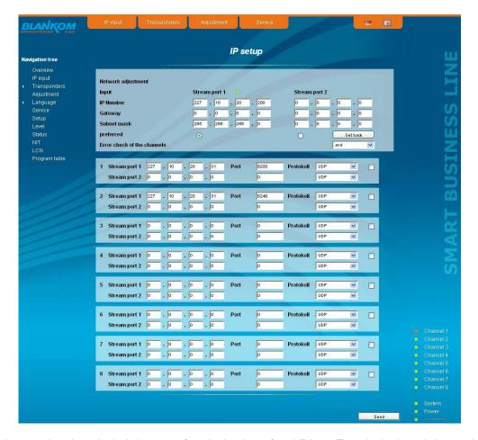
The form of the network settings also includes means for selecting the preferred IP input. The selection is made by pressing the appropriate option button. "Error check of the channels" as described above configures the device for switchover if only one of the monitored channels fails ("or") or only when all monitored channels have failed ("and").
