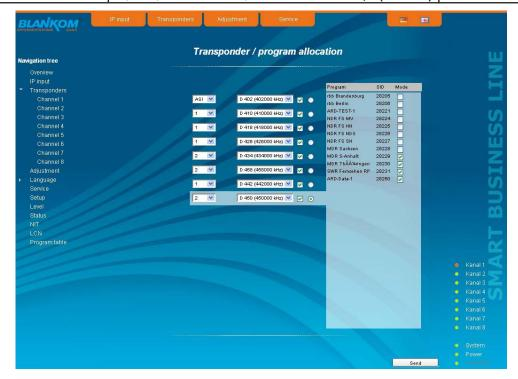
To make changes, first the desired channel is to be selected. This is done either by clicking the appropriate selector outside right next to the output channel in the middle of the channel list or by clicking on "Channel" in the navigation tree on the left side, which is listed as a submenu of the menu "Transponders".
