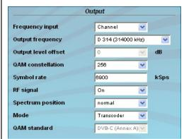
Output (only 5107.01) output parameters of the channel
