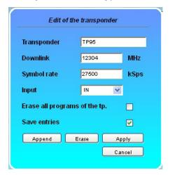
Existing entries can be changed or new ones are attached. By clicking the appropriate box the program list of the transponder can be deleted and changed or additions can be stored into the database permanently. If the box "Save entries" is not clicked, the changes will remain only as long as the user interface is open. With the next start of the user interface the changes are lost. In this simple way, the program data is kept up to date.
