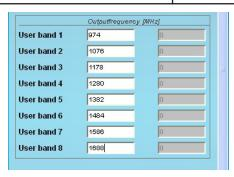
If the point "unicable" is selected for one or both satellite ports, the input mask is expanded by the unicable settings. If only one satellite port is set to unicable, the settings for the other port is disabled and grayed out. For an active unicable port the other settings are inactive and grayed out.
