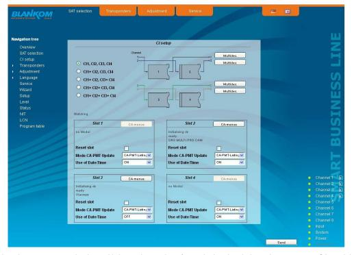
After the selection above one can make the multi-decryption settings for each signal path through one or more CA modules, if necessary. For this purpose the "Multidec" button is to press and leads to the following menu:
