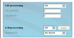
CAT processing CA system ID Operator ID selection: on, on with CA filter, off adjustment range: 0...65535 adjustment range: 0...65535
