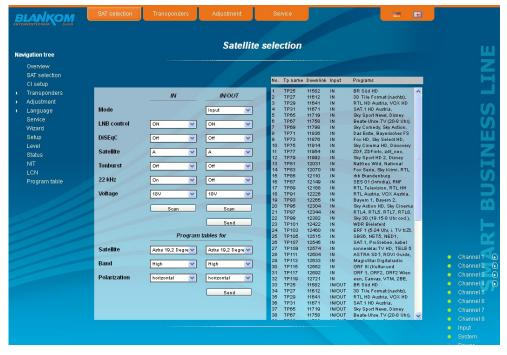
The setting screen is divided into two sections "LNB Control" and "Program tables for", for the two satellite jacks 1 (IN) and 2 (IN/ OUT). The parameters of both sections can be adjusted separately with the "send" button below and then transferred. If the second sat jack (IN/ OUT) is configured as a loop-through output, or not used, then the input configuration parameters of the LNB control and program table are grayed out and not adjustable.
