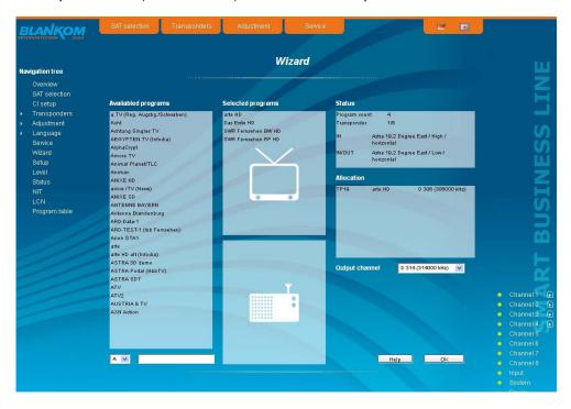
In this way, now up to 8 transponders per A-QAMOS-4CI can be selected to be transferred. First, as the output channel the next higher channel to the last selected program package is offered. But for each packet the output channel can be chosen freely in the total frequency range. If an incorrect selection is made, it can be removed by double-clicking the unwanted selected transponder in the right field.
