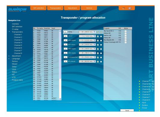
To make changes, you must first select the desired channel. This is done either by clicking the appropriate selector outside right next to the output channel in the middle of the channel list or by clicking "Channel" in the navigation tree on the left side, which is listed as a point of the menu "Transponders".
