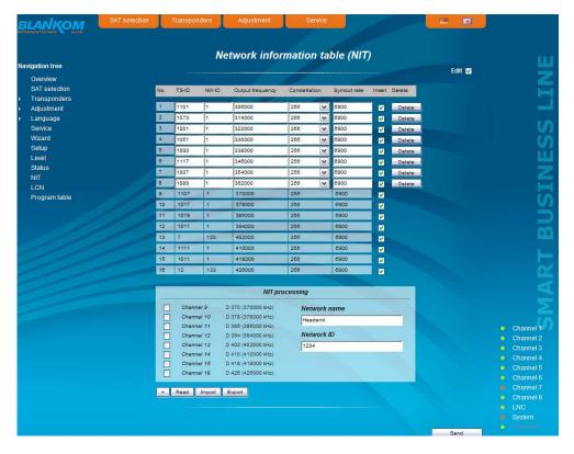
For changes of the NIT is to be noted that these changes must be made in the NIT of each device. It is therefore recommended to prefer the automatic NIT processing of the manual NIT processing.
