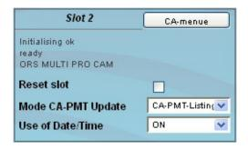
Individual CA modules must be initialized before setting the CA services. For this purpose the box "Reset slot" is clicked. The mode of the CA-PMT update will be adjusted on the next line. You can select between CA-PMT list and CA-PMT entry, where the latter is not supported by all CAM's.
