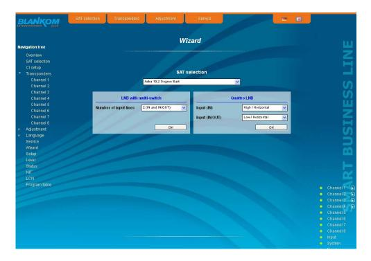
First choose the configuration of the system. If the system is equipped with LNB and multiswitch, so you can select the number of feeds on the left. If the system is operated with a Quattro LNB, so you choose from the right side, which satellite level contact with the corresponding input jack. By pressing the "OK" button, the corresponding data are loaded and you will be forwarded to the selection of the channel or transponder.
