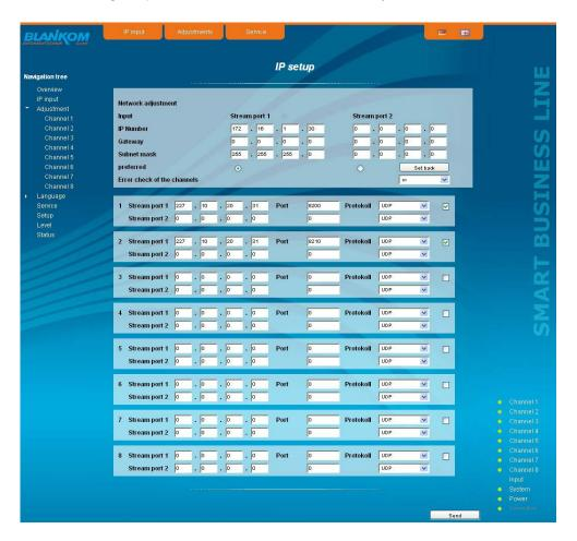
The form of the network settings also includes means for selecting the preferred IP input. The selection is made by pressing the appropriate option button. "Error check of the channels" as described above configures the device for switchover if only one of the monitored channels fails ("or") or only when all monitored channels have failed ("and").
